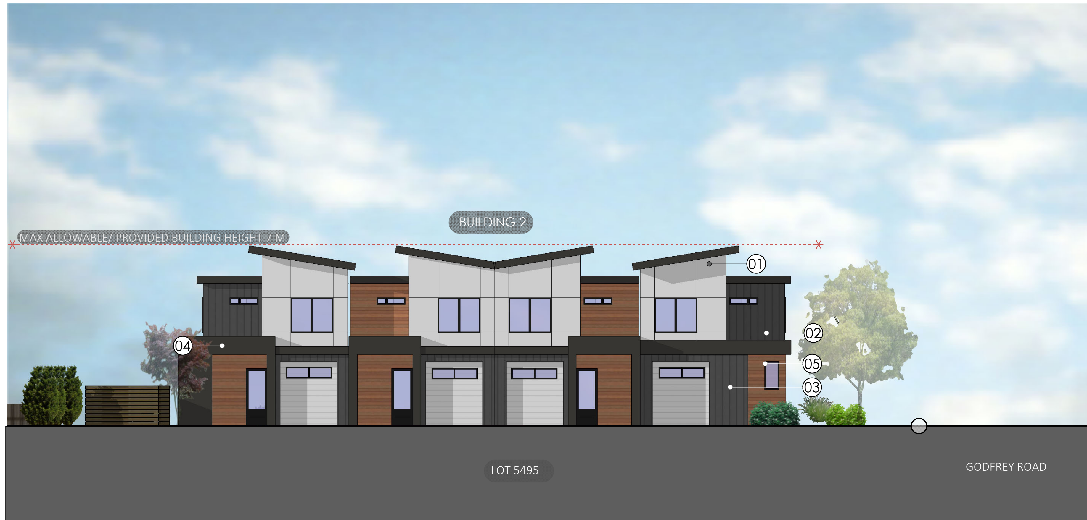
NORTH ELEVATION | TOWNHOMES | BUILDING 2 REAR ELEVATION | Scale 1/8" = 1' |
